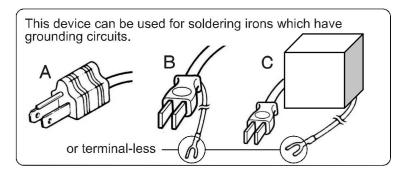
Soldering irons which have no grounding circuits are not applicable.
