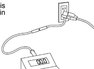
6 Turn on the soldering iron and wait until the tip is heated. Then tin the tip with a small amount of solder.
