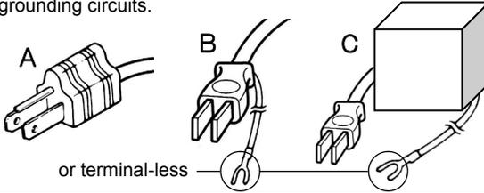
Soldering irons which have no grounding circuits are not applicable.
