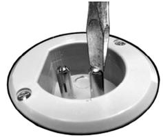
To be loose, narrow the gap of the contact pins on the sensor base with pliers and such.
