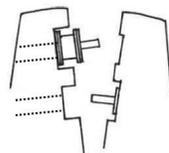
2 Close the handles to insert the chain rivet checking that the links are in the groove correctly. Finish the work after check that the chain rivet is pierced over the opposite plate.
