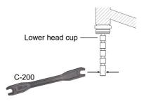
Gently turn the handle clockwise. Continue to cautiously turn the handle until both head cups meat to the edges of the head tube. Turn the handle still more ensuring the head cups advance into the head tube straight. Cautiously turn the handle during the operation to prevent cups are installed diagonally.
