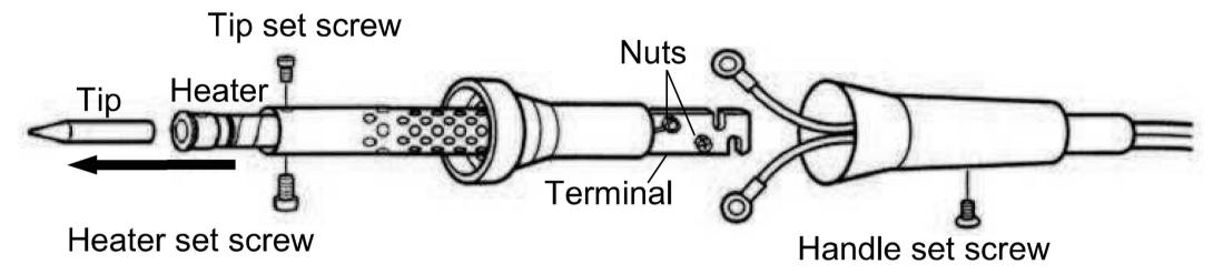
4 Reset the new heater and assemble the soldering iron as it was before.
