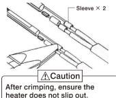
6 Set the heater, lead of the heater, and power cord as shown.
