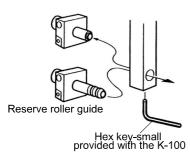
We have installed the roller guide which is applicable to cut while cooling with water on the recently manufactured K-100. Use without replacing the roller guide just as it is. But if the roller guide of your K-100 is not for watering, in other words, cannot let run water through internally, replace the roller guide with the reserve roller guide provided with this product the K-105.
