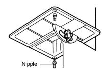
Insert the two nipples provided into the two threaded holes on the underside of the table of the K-100 as shown in the illustration.
