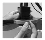
6 Install the LED ring light at the barrel securing the three screws.
