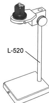
Please exchange the post of the standard table to the long post when use the optical lens singly without the ring since the working distance becomes long.
